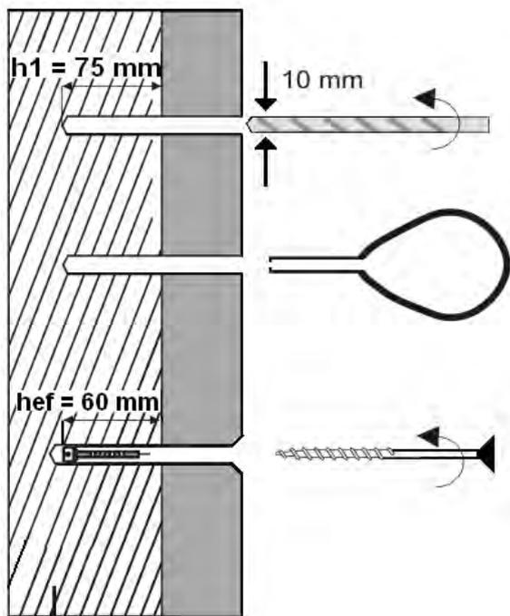
Drill the bore hole perpendicular to the surface of the base material considering the drill method given in Table 9 and 10
