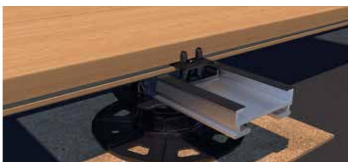
Hidden fastening using deck gliders twin system clip
