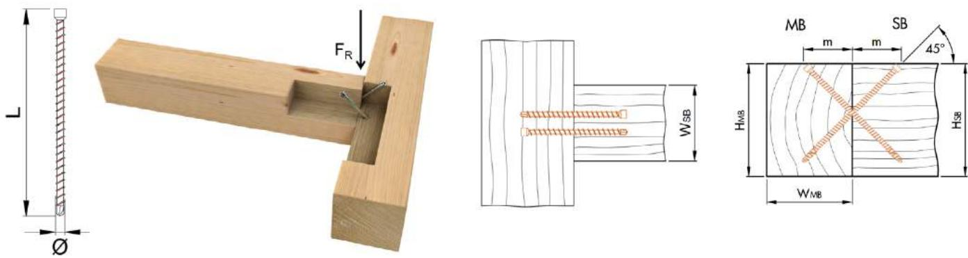
Load-carrying capacity of screws with minimum required lengths.
