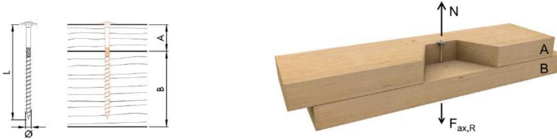
Axial load-carrying capacities of screws with minimum required lengths.
