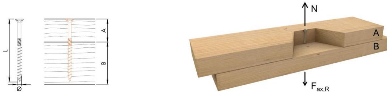
Axial load-carrying capacity of screws with minimum required lengths.
