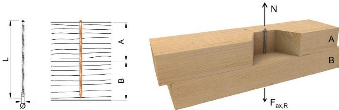
Axial load-carrying capacities of screws with minimum required lengths.
