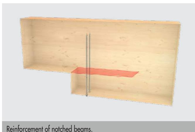
Reinforcement of notched beams.
