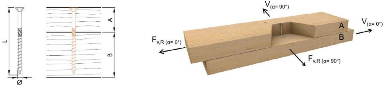
Axial and lateral load-carrying capacities of screws with minimum required lengths.
