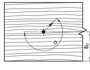
**Notes:** The minimum distances for lateral load-carrying screws are based on EN 1995:2014 considering a softwood density of  $\rho_k \leq 420 \text{ kg/m}^3$ , where  $d$  = nominal screw diameter. For timber-to-timber joints, the axial distances of  $a_1$  and  $a_2$  must be increased by 1,43.
