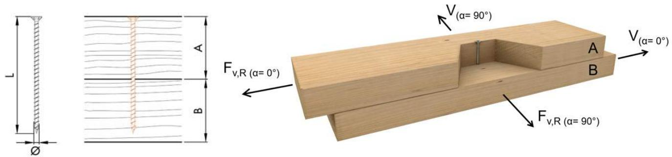
Lateral load-carrying capacities of screws with minimum required lengths.
