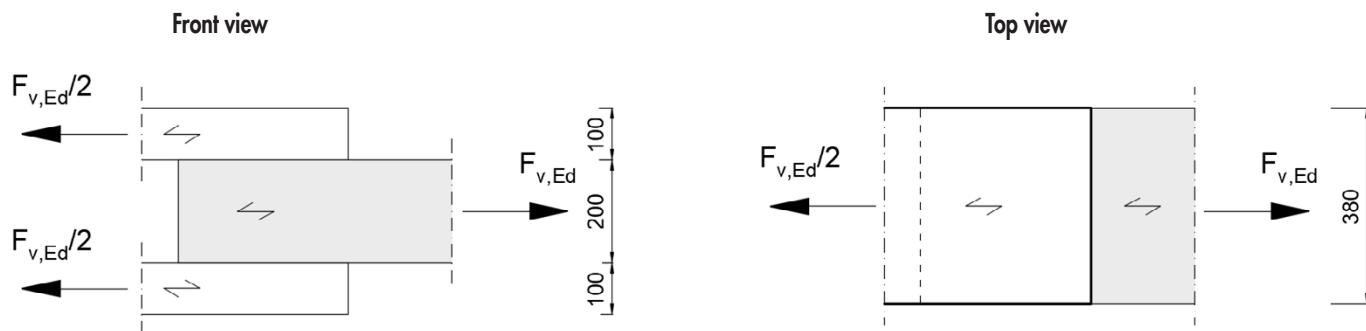
→ to KonstruX ST ZK Design Tables, load carrying capacity of shear-tension screws, with  $A = h_s = 100 \text{ mm}$
