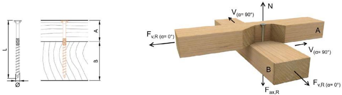
Axial and lateral load-carrying capacities of screws with minimum required lengths.
