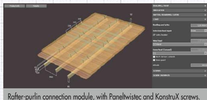
Rafter-purlin connection module, with Paneltwistec and KonstruX screws.
