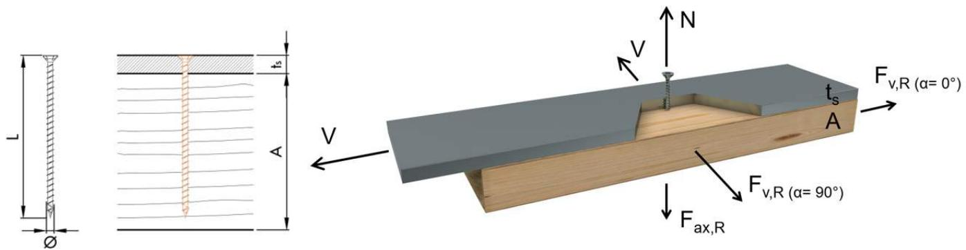
**Load-carrying capacities of screws with minimum required lengths.**
