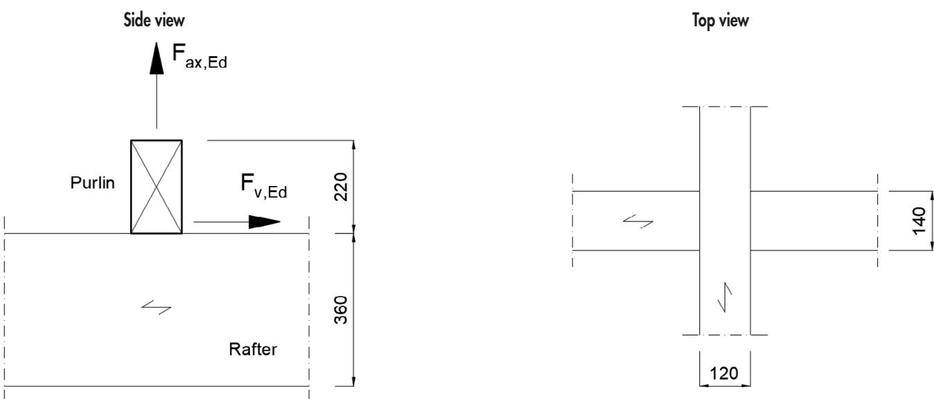
→ to Paneltwistec AG SK Design Tables, axial load-carrying capacity, with  $A = h_p = 220 \text{ mm}$
