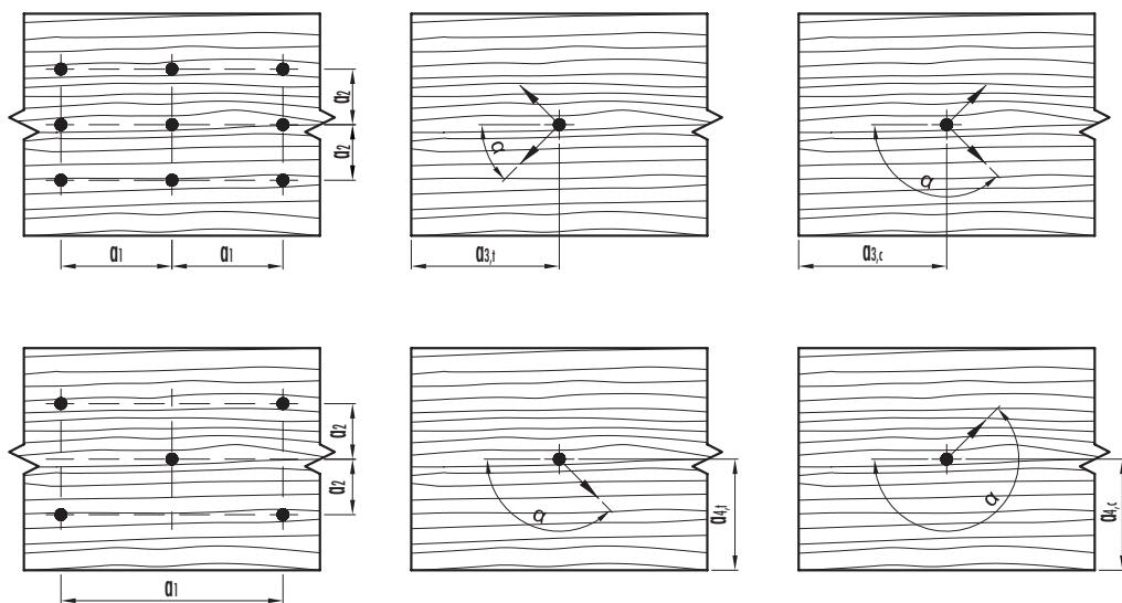
**Notes:** The minimum distances for lateral load-carrying screws are based on EN 1995:2014 considering a softwood density of  $\rho_k \leq 420 \text{ kg/m}^3$ , where  $d$  = nominal screw diameter. For timber-to-timber joints, the axial distances of  $a_1$  and  $a_2$  must be increased by 1,43.
