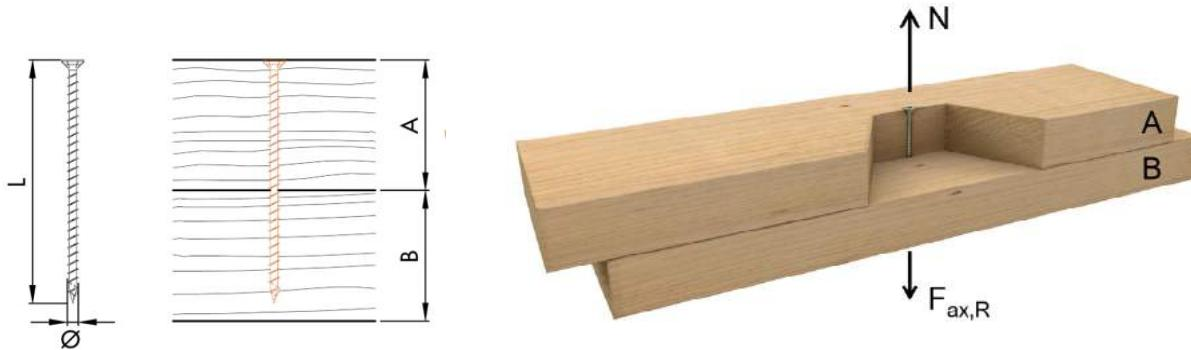
Axial load-carrying capacities of screws with minimum required lengths.
