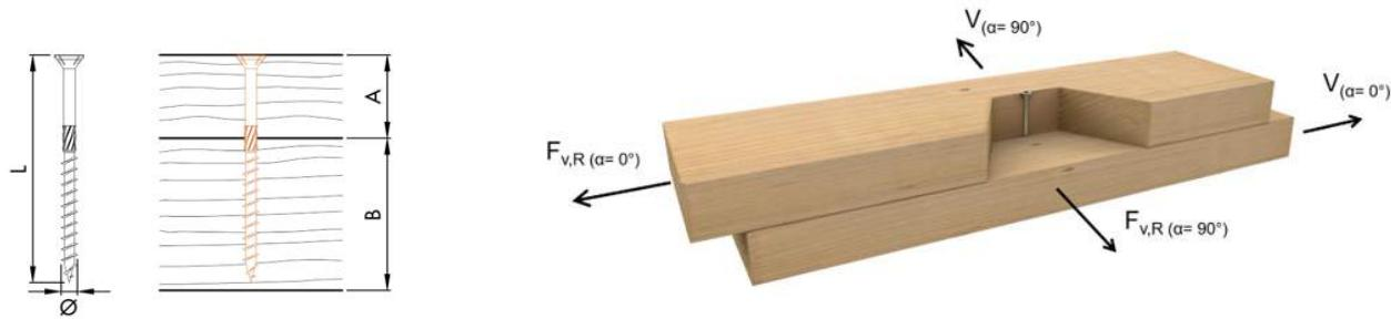
Axial and lateral load-carrying capacities of screws with minimum required lengths.
