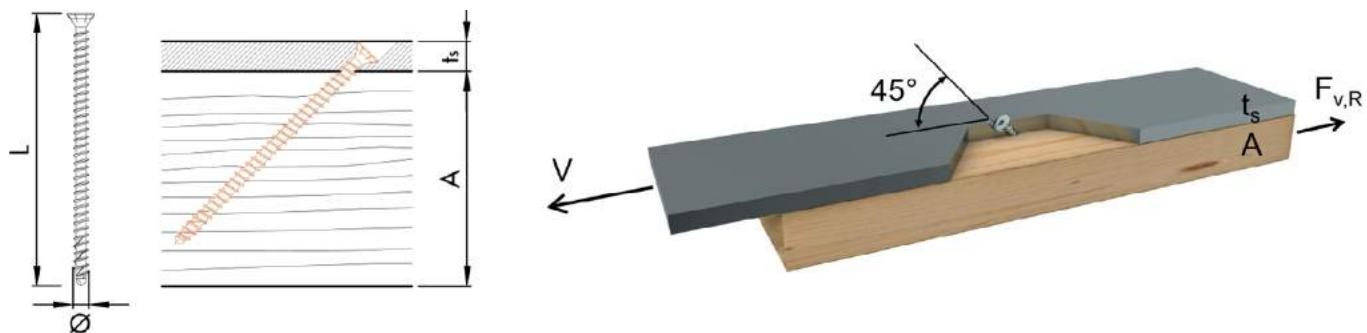
Load-carrying capacity of shear-tension screws with minimum required lengths.
