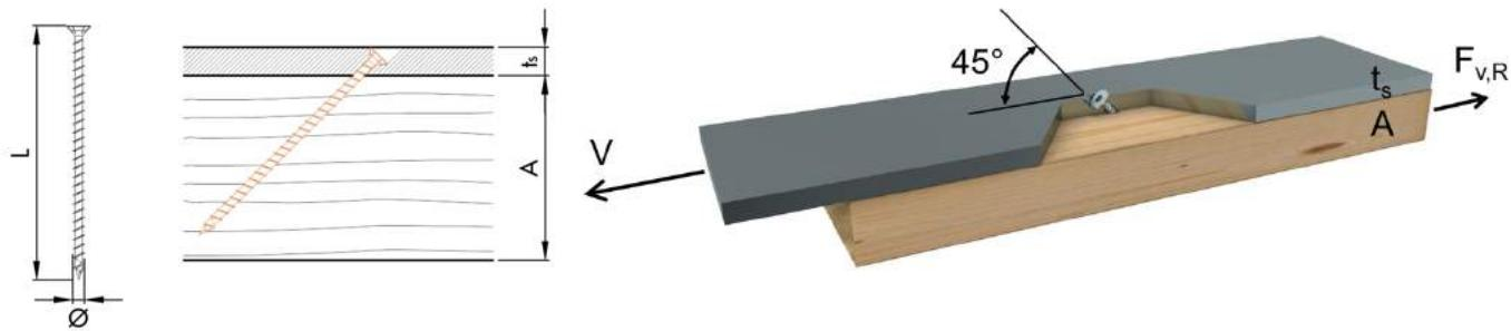
Load-carrying capacity of shear-tension screws with minimum required lengths.
