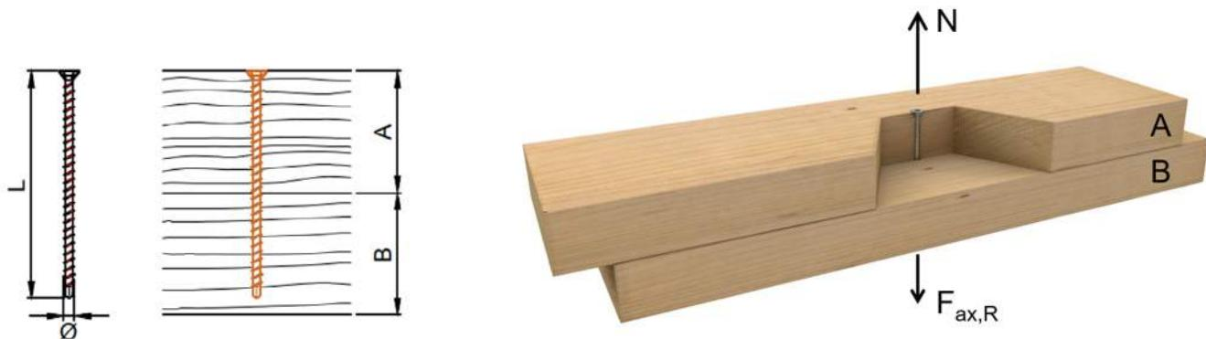
Axial load-carrying capacity of screws with minimum required lengths.
