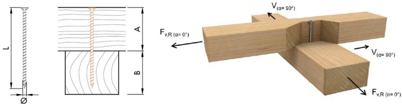
Lateral load-carrying capacities of screws with minimum required lengths.
