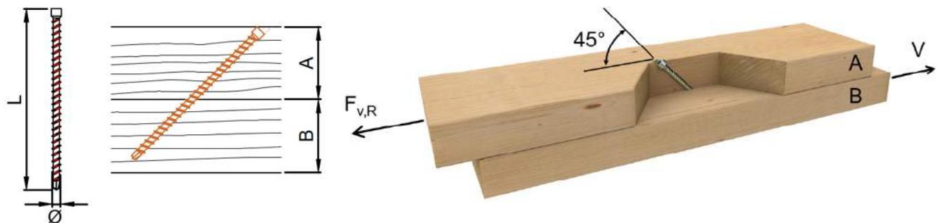
Load-carrying capacity of shear-tension screws with minimum required lengths.
