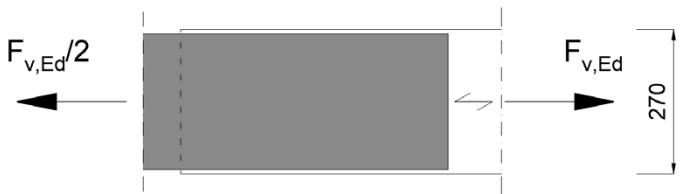
→ to Paneltwistec AG SK Design Tables, lateral load-carrying capacity, with  $A = w = 100 \text{ mm}$ ,  $t_s = 3 \text{ mm}$  (thin plate)
