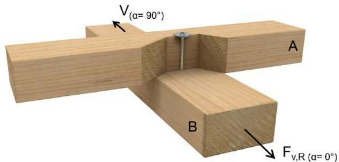
Lateral load-carrying capacity of screws with minimum required lengths.
