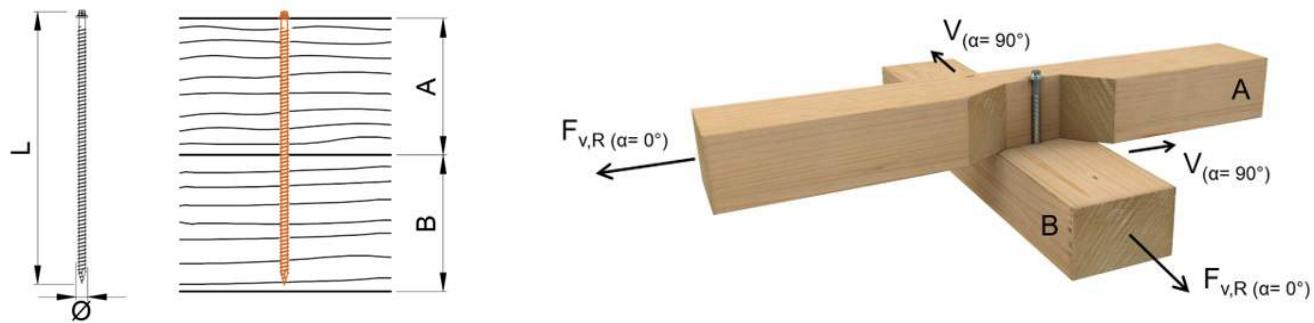
**Lateral load-carrying capacities of screws with minimum required lengths.**
