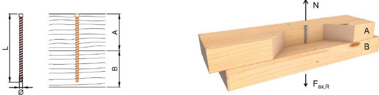
Axial load-carrying capacity of screws with minimum required lengths.
