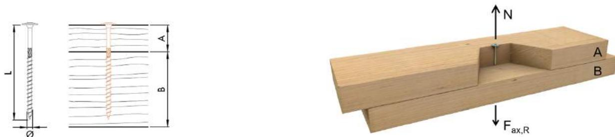
Axial load-carrying capacity of screws with minimum required lengths.
