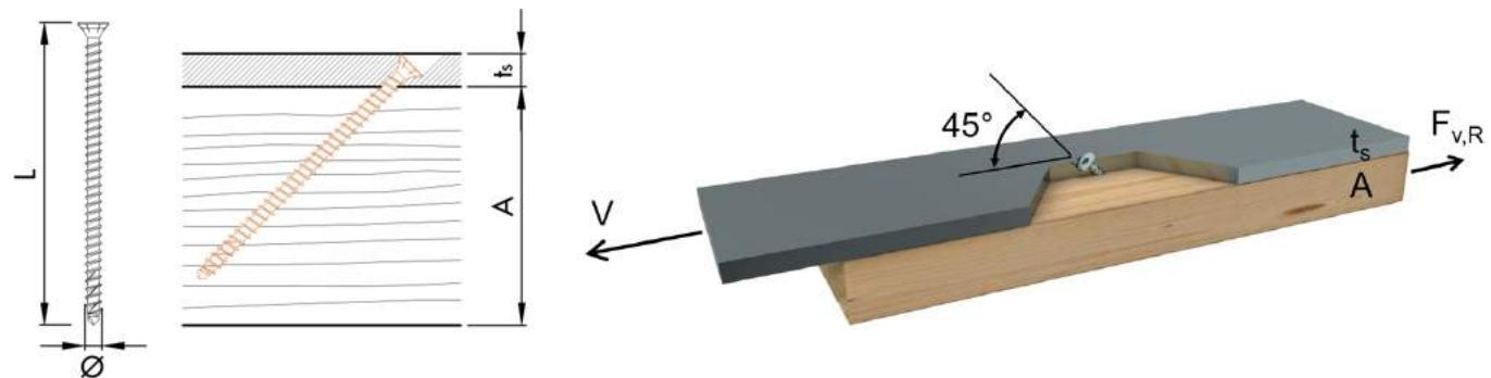
Load-carrying capacity of shear-tension screws with minimum required lengths.
