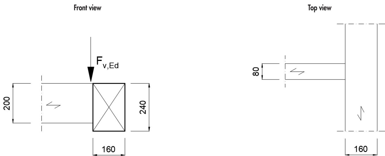
→ to KonstruX ST Design Tables, load carrying capacity of screw crosses, with  $F_{v,Rd} \geq 9,2 \text{ kN}$
