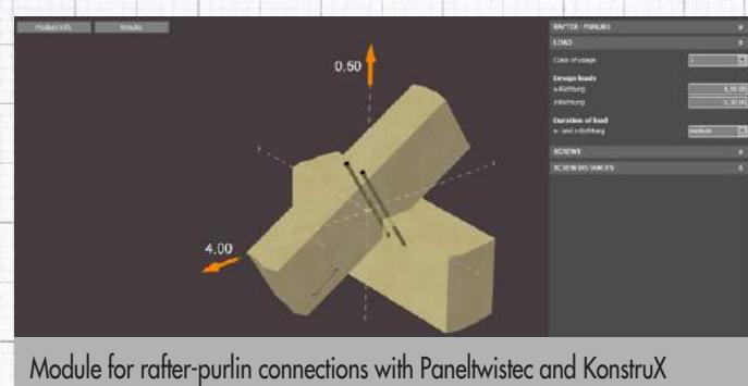
Module for rafter-purlin connections with Paneltwistec and KonstruX
