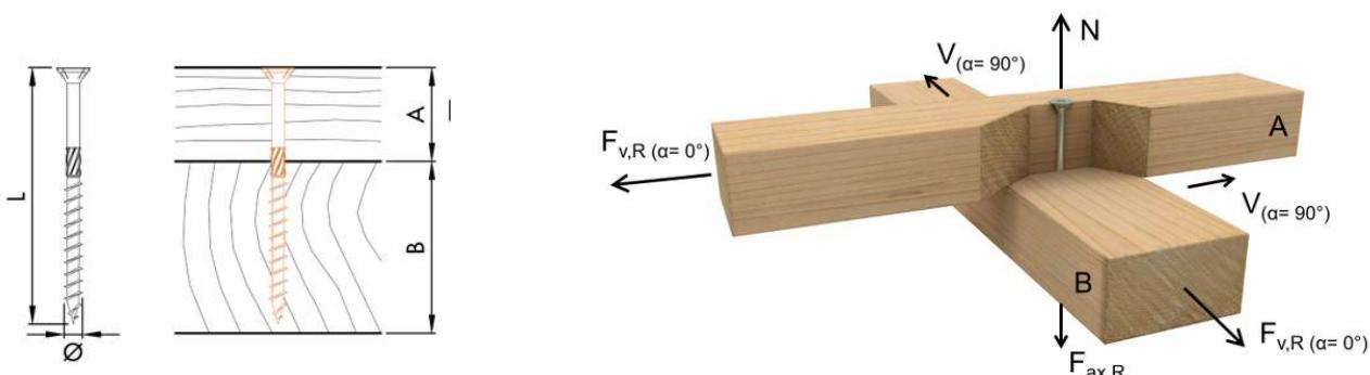
Axial and lateral load-carrying capacities of screws with minimum required lengths.
