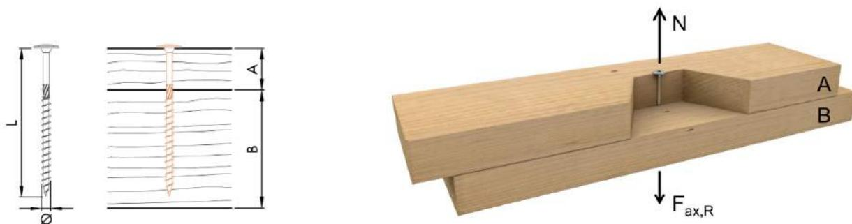
Axial load-carrying capacity of screws with minimum required lengths.
