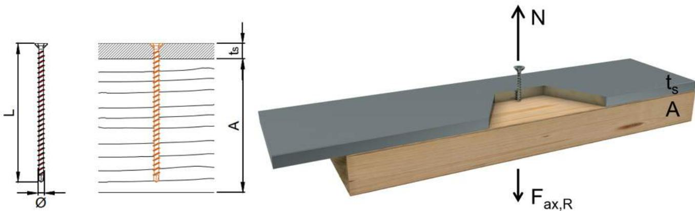
Axial load-carrying capacity of screws with minimum required lengths.
