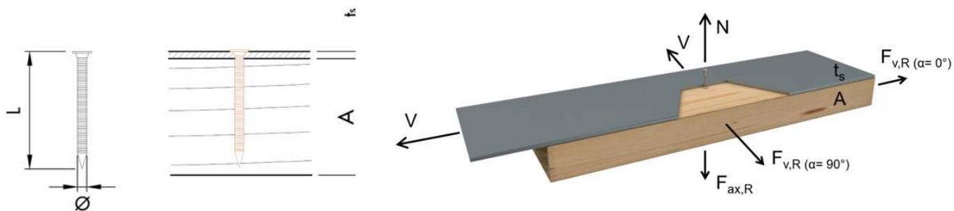
Load-carrying capacities of screws with minimum required lengths.
