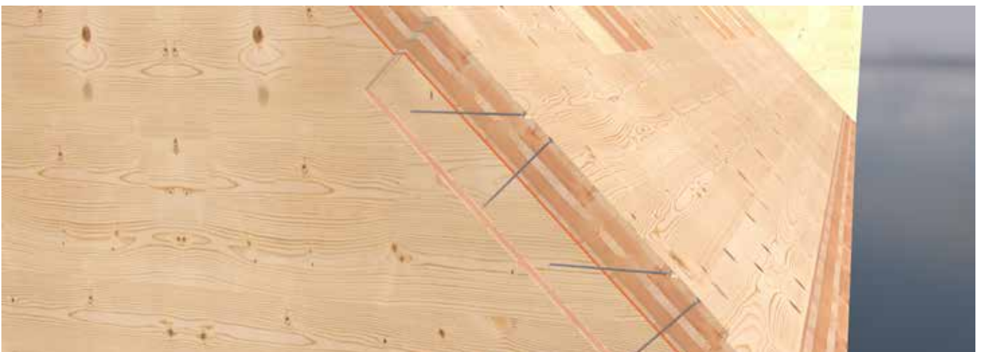
Connection of roof- and wall elements.
