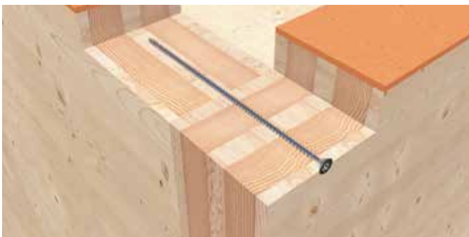
KonstruX in order to connect two walls with each other.
