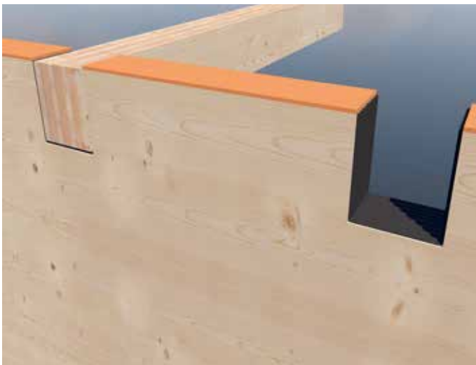
Application of the Silent EPDM decoupling profile under beams for sound insulation between wooden components.
