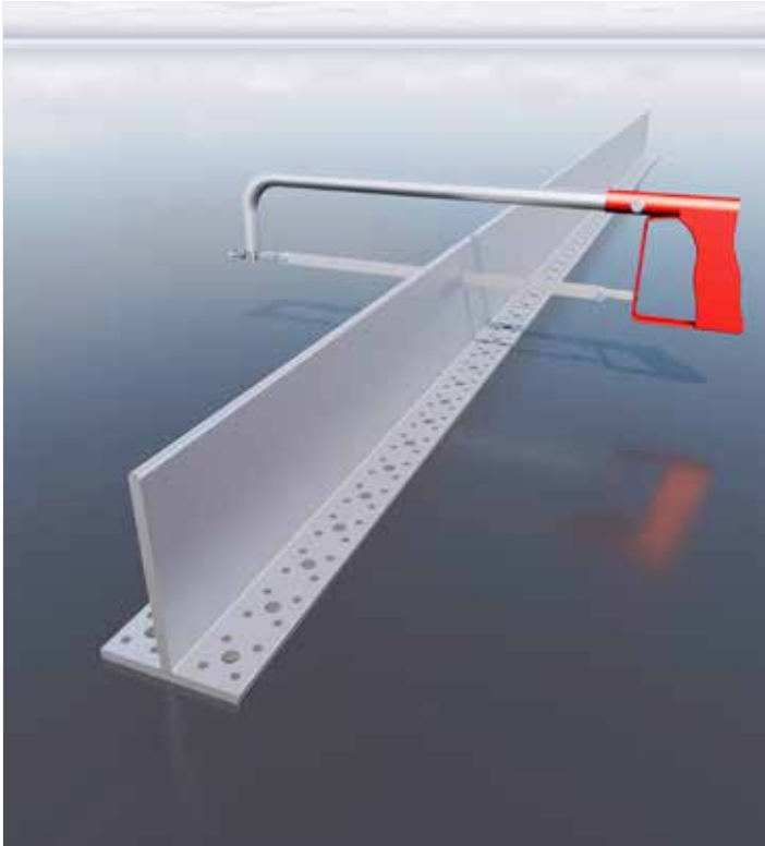
Individual cutting of the profile to length
