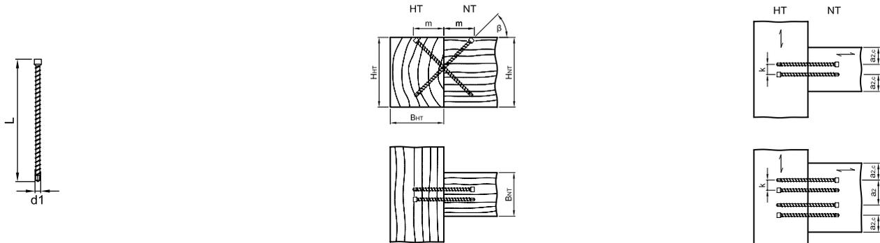
$\alpha_2 = \text{min. } 40 \text{ mm}, \alpha_{2,t} = \text{min. } 24 \text{ mm}, k = \text{min. } 12 \text{ mm}$
