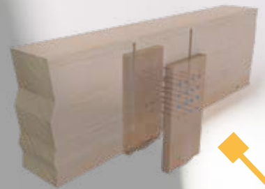
LATERAL BUTT STRAP JOINT
