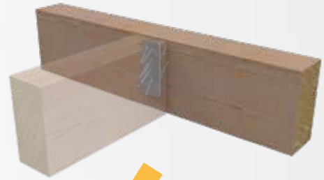
MAIN-SECONDARY BEAM CONNECTION
