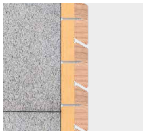
Wall connection with ZK façade screw
