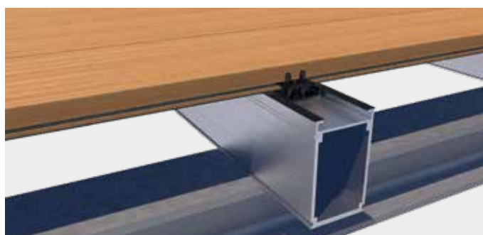
Hidden fastening using deck gliders twin system clip
