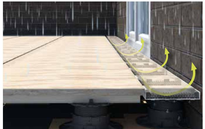
The Draintec adapter allows rainwater to drain away in a controlled manner, with additional back ventilation arising at many detailed points.
