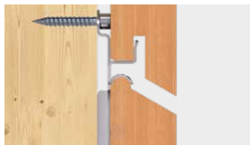
Wall connection with rhombus façade clip
