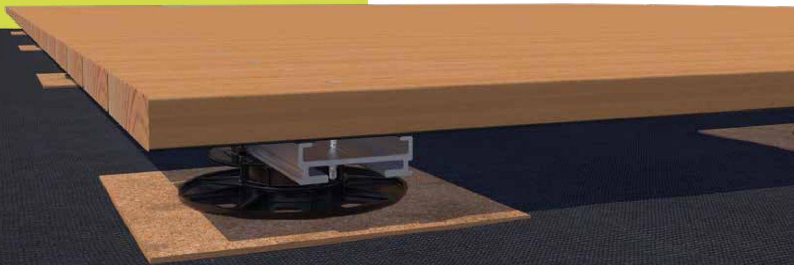
Visible fastening using profile drilling screw
