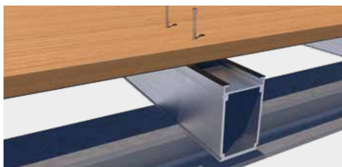
Visible fastening using profile drilling screw
