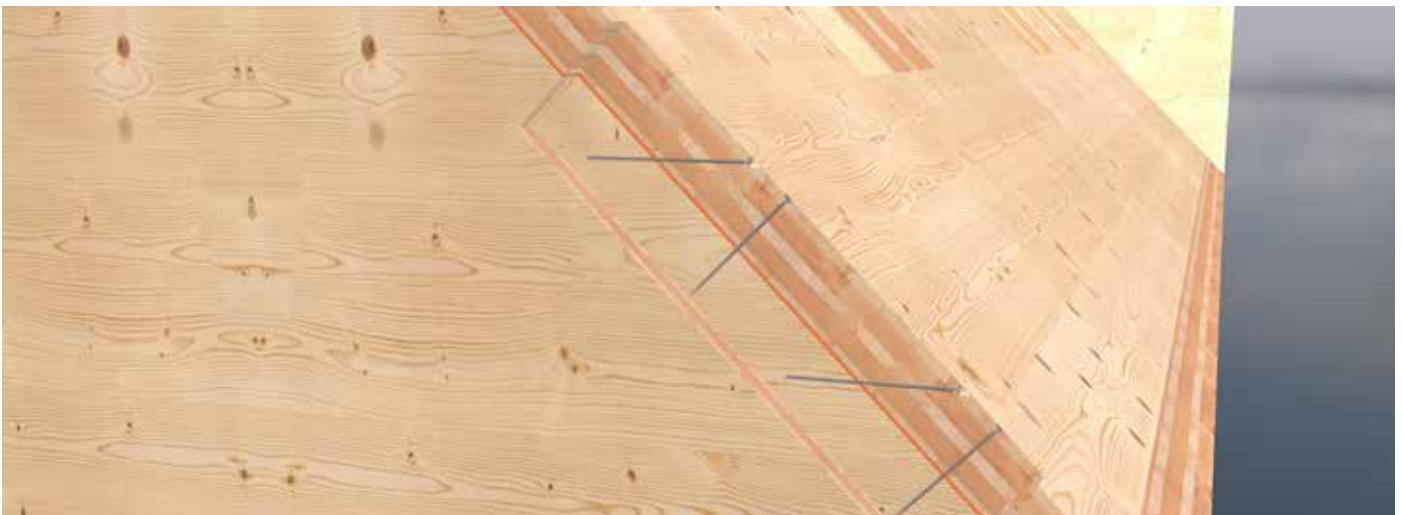
Connection of a roof and wall element
