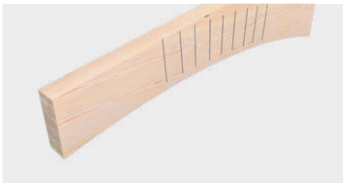
Reinforcement of trapezoidally shaped beams
