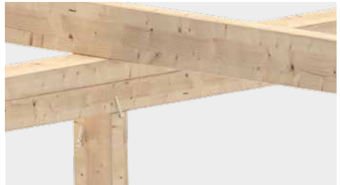
Fastening of supports in timber frame constructions
