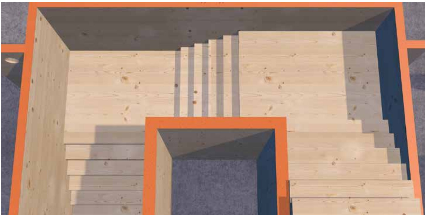
Attach steps to the top of the step support.
