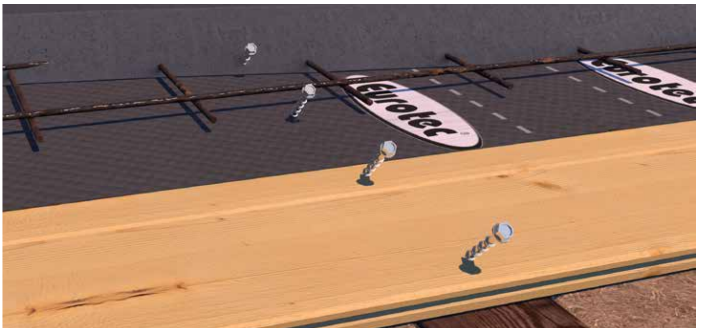
Impact sound decoupling and screed on the TCC ceiling
