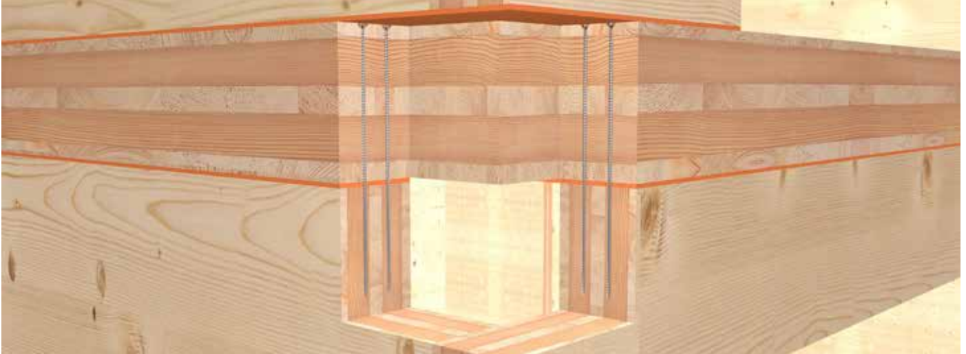
Connection of a wall element and ceiling element
