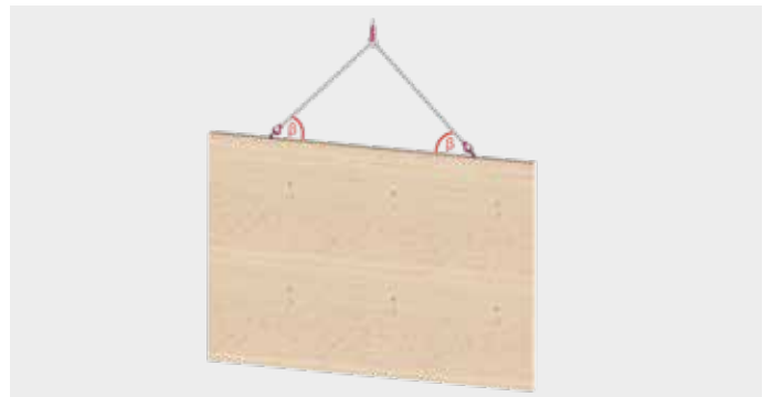
Vertical CLT wall or beam
