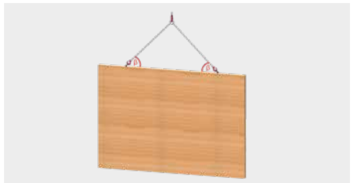
Vertical GLT wall or beam, grain flow: horizontal
