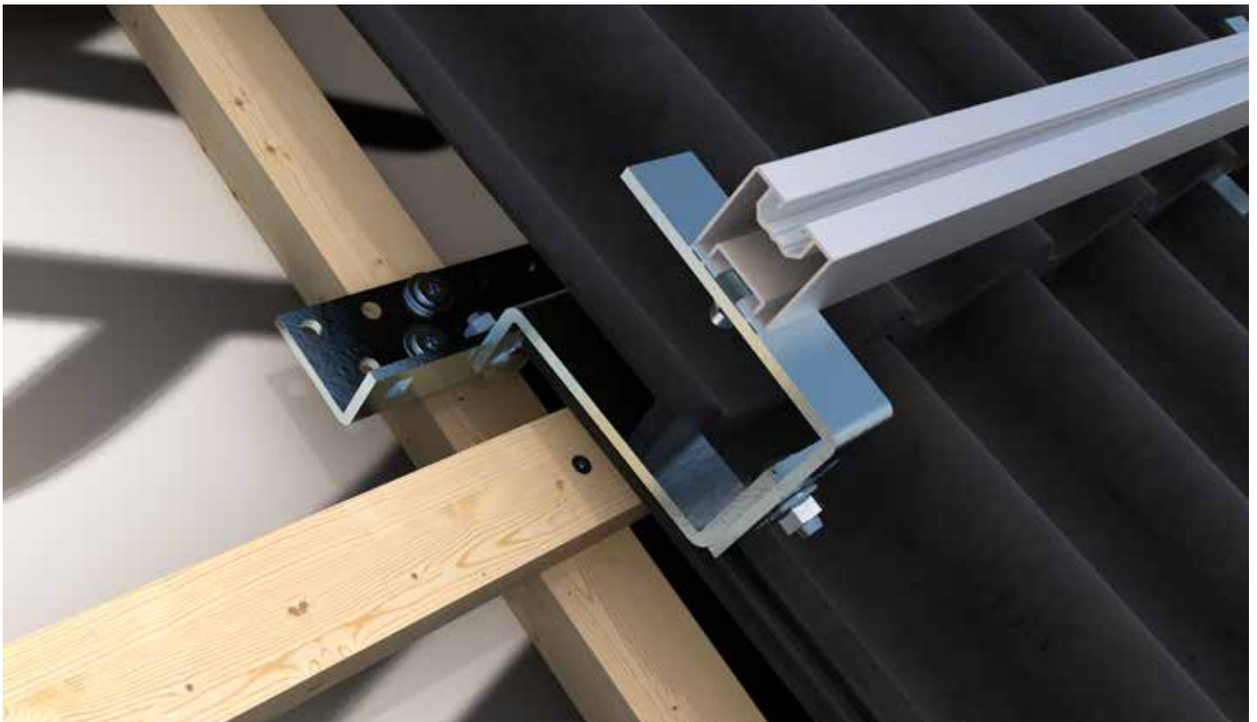
STEP 1: The first step is to screw the roof hook onto the counter-batten with the Topduo or Paneltwistec screws, depending on the roof structure.
