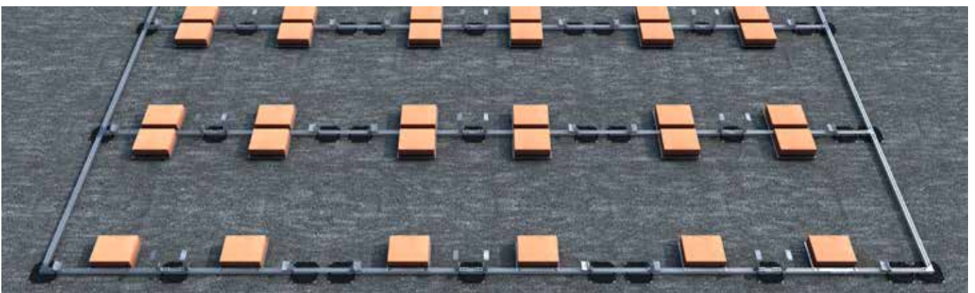
STEP 3: The various joints are screwed onto the profiles.
