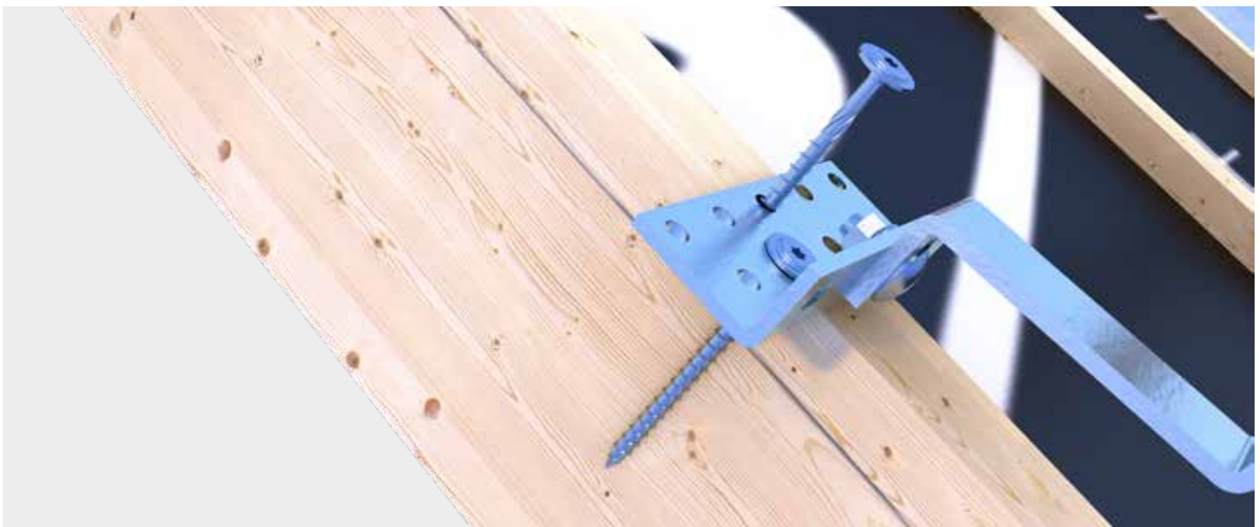
The Paneltwistec washer head screw is used to fasten the roof hook and is screwed into the rafters through the counter-batten.
