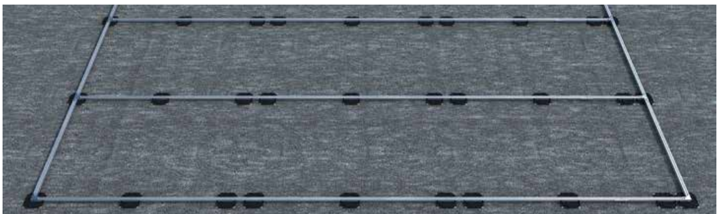
STEP 1: The load distribution plates are arranged with the correct spacing and fitted with installation profiles connected with T- and corner connectors.
