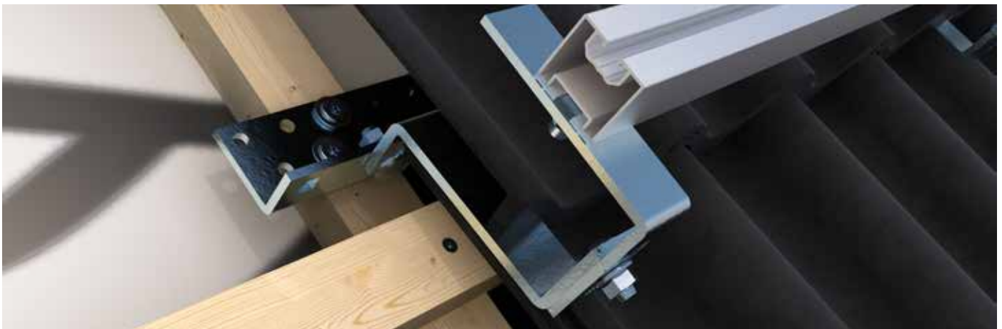
Roof hook FLEX installed on the counter-batten, guided through the released roof tile, with pitched roof installation profile installed.
