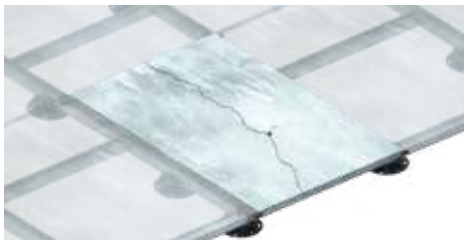
Increased risk of breaking individual slabs due to a lack of support profile.
