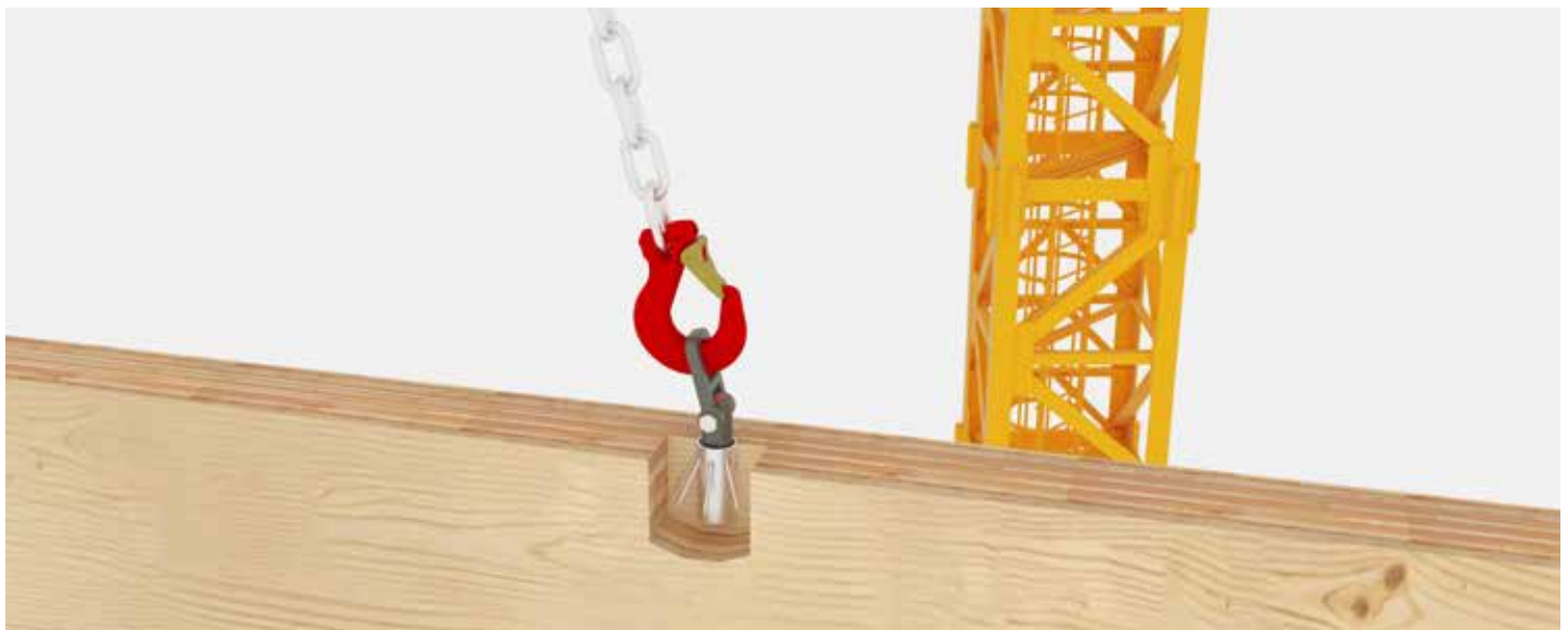
Application of lifting anchor to transport a wall.
