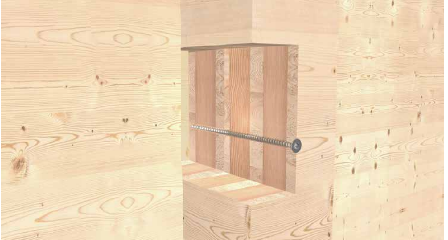
Connection of a wall and a support for the ceiling joist.
