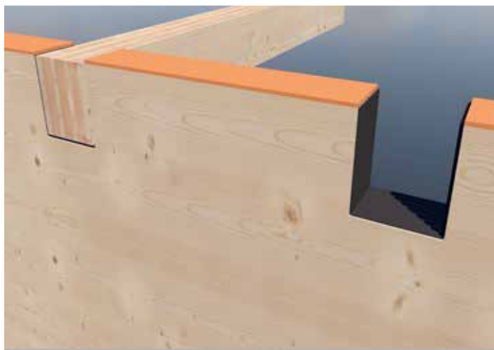
Application of the Silent EPDM decoupling profile under beams for sound insulation between wooden components.
