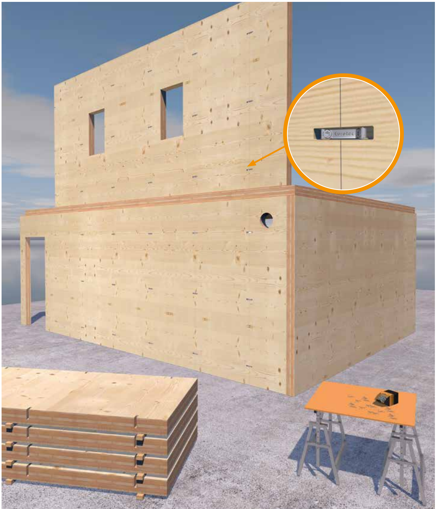
Unevenness compensation through screws and edges
