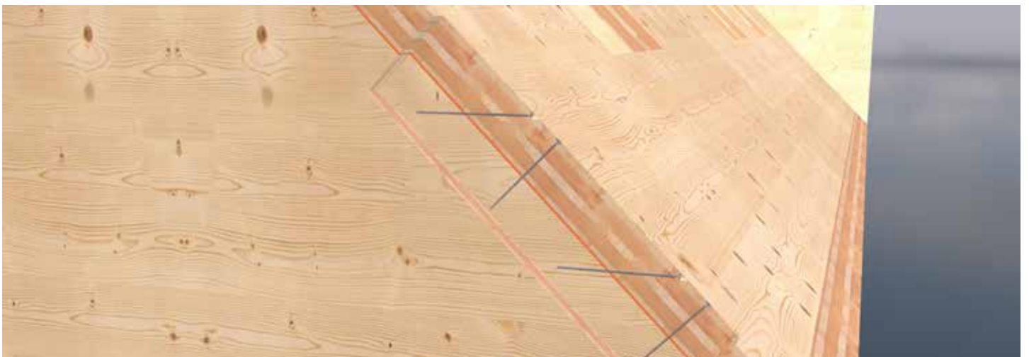
Connection of roof- and wall elements.
