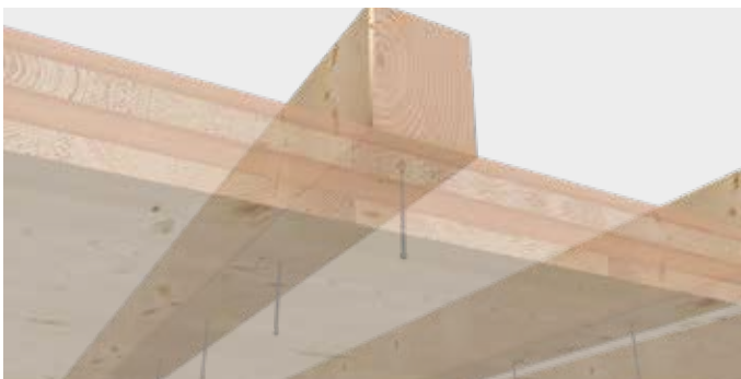
KonstruX DUO for fastening a downstand beam
