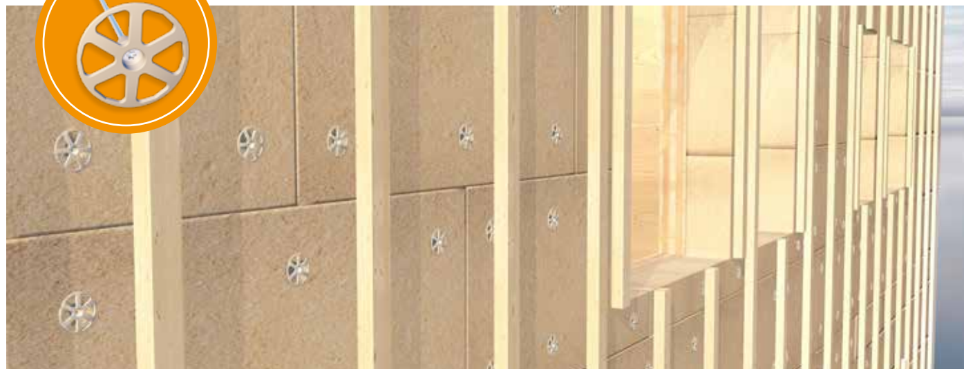
Klimax for fastening insulation material.
