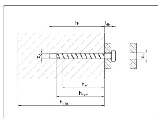
Rock hexagon head and hexagon head with flange: sizes 7,5, 10,5 and 12,5
