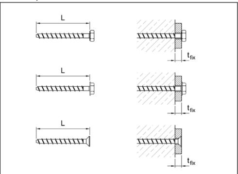
Table B4: Screw length and maximumum thickness of fixture  $t_{fix,max}$
