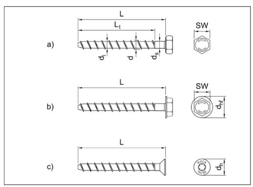
**Screw types:** a) Rock hexagon head 7,5, 10,5 and 12,5. b) Rock hexagon head with flange 7,5, 10,5 and 12,5. c) Rock countersunk head 7,5. Head marking: "Rock" and size x screw length.
