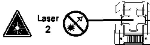
The cross-line laser generates a visible laser beam that emerges from the front of the device. It is a class 2 laser product according to IEC60825-1: 2014 "Radiation safety of laser products" Class 2 laser products. Do not stare directly at the laser beam and do not point it unnecessarily at other people. The eyes move away or instinctively blink for protection.
