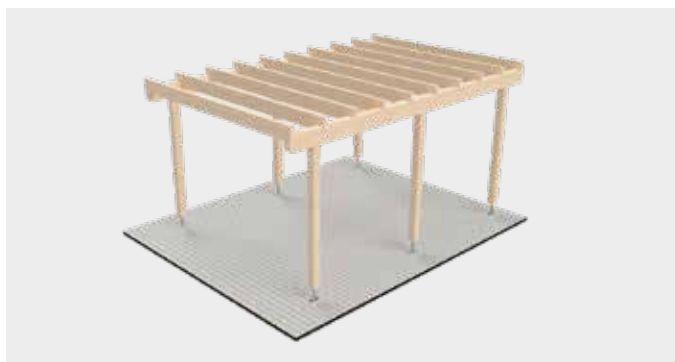
Design-based wood preservation in a carport with PediX Easy.
