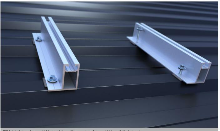
STEP 1: In the first step, the trapezoidal sheet installation profile is screwed onto the trapezoidal sheet with thin sheet metal screws.
