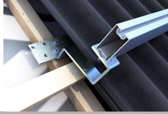
Pitched roof installation profile 40 x 40/40 x 80 fastened to the roof hook by means of the hammer head screw and locking nut.
