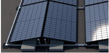
STEP 4: Starting with the first module field row, you can now place the solar modules on the module uprights and fix them with module clamps.
