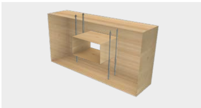
Reinforcement of beam openings
