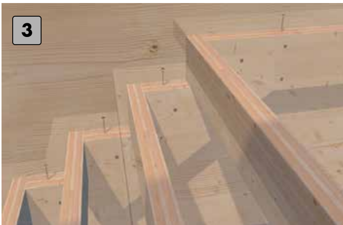
Attach steps to the top of the step support.
