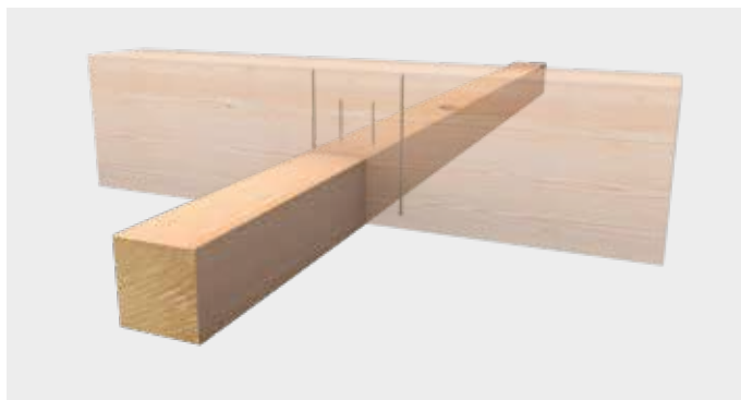
Reinforcement of the main/secondary beam supports
