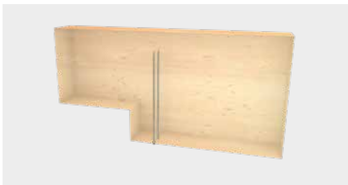
Reinforcement of notched beams
